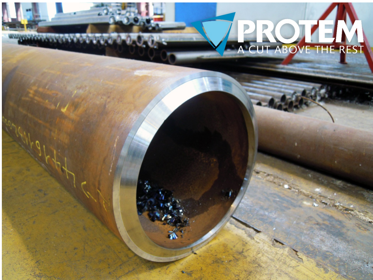
Figure 1 - Compound bevel made with a high speed beveling bench PROTEM BB3-16
