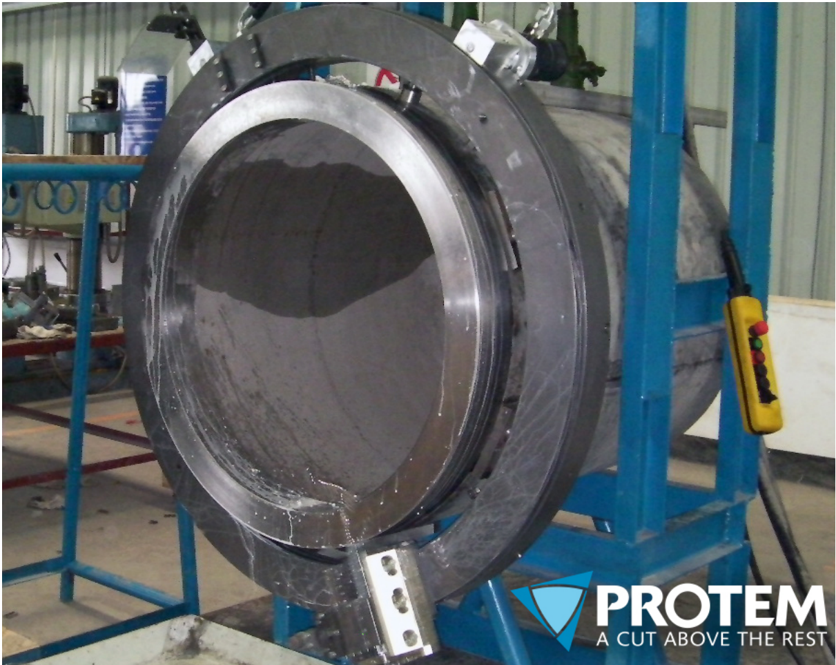
Figure 11 - Figure 6- PROTEM clamshell TTNG1016. 32”-40” heavy wall thickness – Material : Austenitic stainless steel
